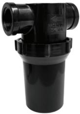
The DEMA #50.41.1 3/4" NPT strainer is an in-line 200 mesh (80 microns) strainer recommended for all MixRite installations. The in-line strainer will keep debris out of the MixRite unit, increasing the life of the seals.
